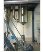
**Spray Dryer:** Spray drying unit is also installed as a part of dairy unit for production of milk powder from liquid milk. It is a quick drying process utilizing hot air for drying of atomized liquid droplets.
