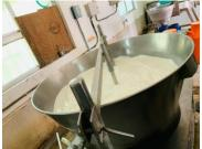
**Khoa making machine:** A batch type mechanically agitated khoa making machine having a capacity of 120 Litres is installed in the unit for rabadi/khoa preparation. Continuous stirring prevents charring of the milk.
