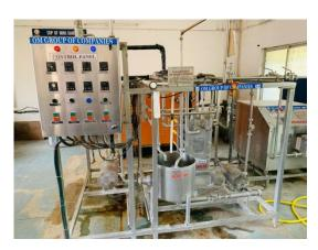
**Pasteurization unit:** Pasteurization inactivates some undesirable enzymes and reduces number of many spoilage bacteria resulting in increase in shelf life of the milk up to 2-16 days depending upon the processing condition, type of packaging and storage conditions. A continuous plate pasteurizer based on high temperature short-time (HTST) method is used for pasteurization. Other than this, storage tank, boiler, chiller and homogenizer are part of the whole pasteurization assembly.
