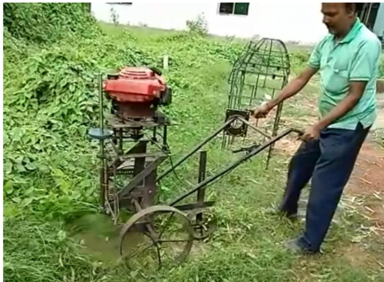
Figure 2. Photograph of residue cutter
