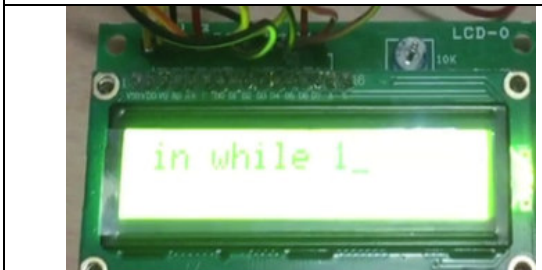
Fig 10: Waits for Ultrasonic Sensor to Trigger
