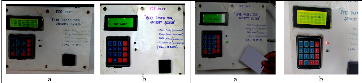
Fig 11:a) Entered Password, b) Displayed Door Closed
