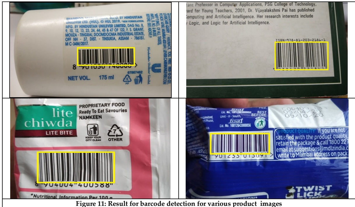
Figure 11: Result for barcode detection for various product images
