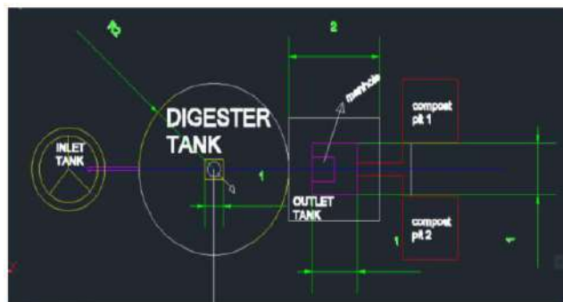
Plan of the Biogas plant
