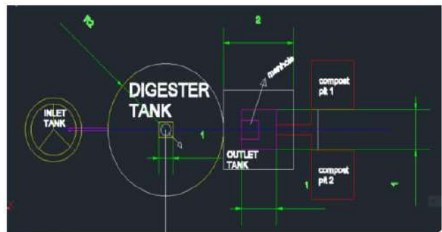
Plan of the Biogas plant
