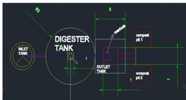
Plan of the Biogas plant
