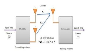
The channel capacity has not really increased because we still have to transmit two signals at a time 2.The MISO capacity is given by,
