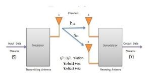
The channel capacity has not increased. The multiple receive antennas can help us get a stronger signal through diversity. The SIMO channel capacity is given by,
